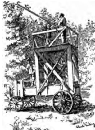
2377. Square tower, giving more working space for the nozzle-men than the conical form.
